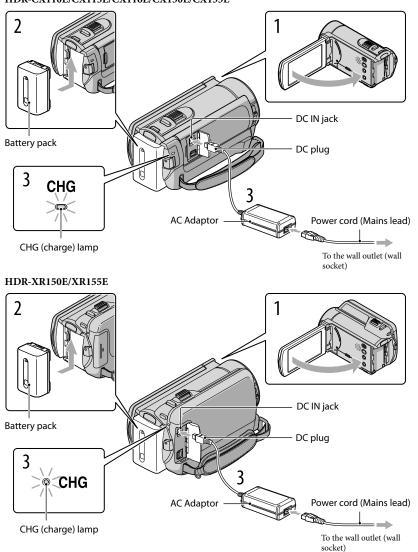
You can charge the "InfoLITHIUM" battery pack (V series) after attaching it to your camcorder.
